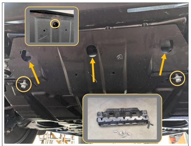
15. Remove the front skid plate by removing the 5x 14mm hex bolts securing it to the chassis. Retain the bolts for use later.
