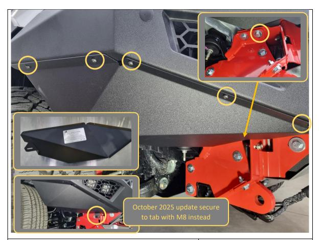
130. Temporarily remove the 2x M10x30 hex bolts from the impact assemblies in preparation for fitting the bash plate. Set them aside.
