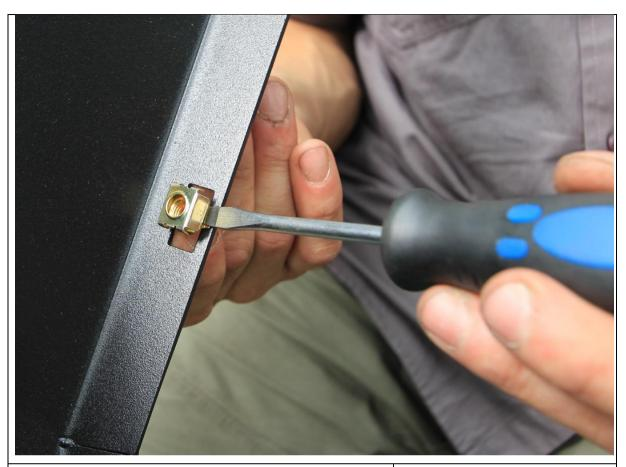
87. Fit 10x M6 cage nuts into the rectangular slots in bottom of wing (5x per side)
