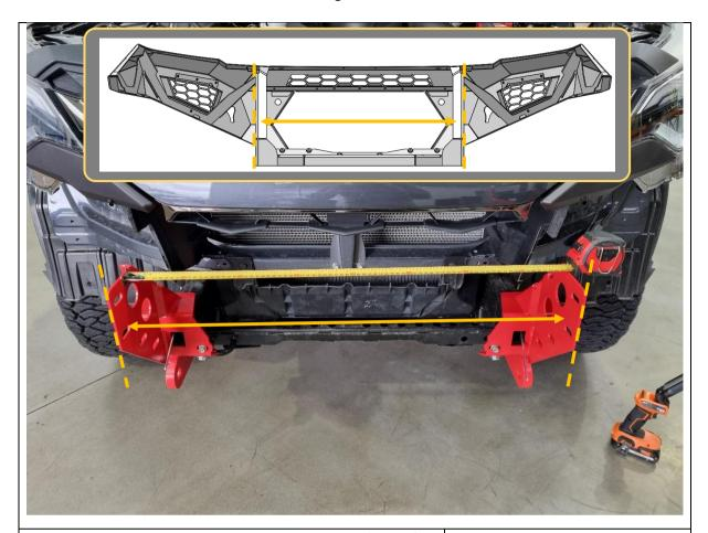
76. Measure the distance between the outside faces of uprights on bar using tape measure. Write distance below for reference if required.
