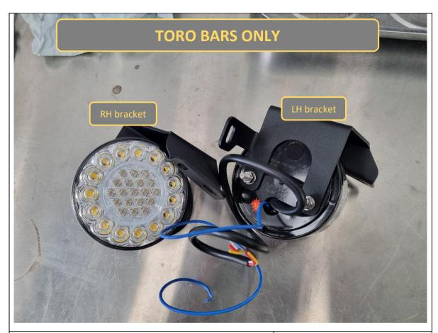
83. **Toro only.** Fit indicator units to the indicator mounting bracket, using fasteners supplied with the indicator.
