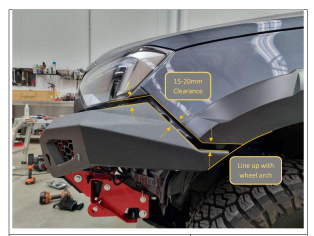
115. With assistance, from another person, align the bar with the edges of the vehicle. Adjust such that the clearances are neat, and the bar is symmetric left/right on the vehicle.
