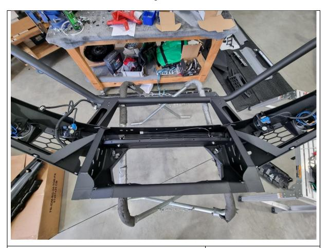
90. Route the bumper wiring harness through the inside of the bullbar.
