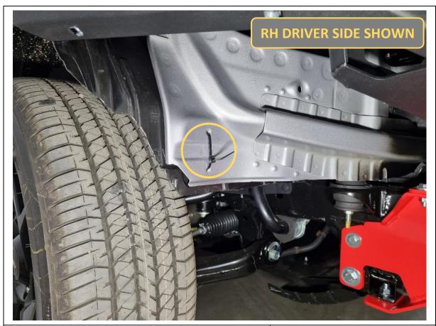
137. **Optional.** Drill a hole through the inner wheel arch liner and use a cable tie to secure it to the body, as shown.
