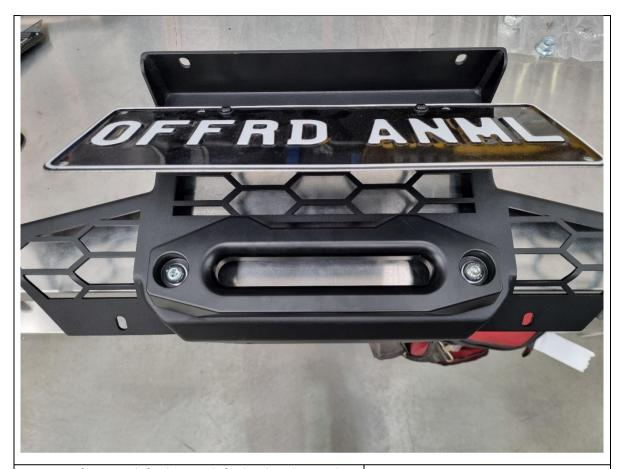
122. If required, fit the winch fairlead to the mesh fairlead mount using M10 or 3/8" fasteners supplied with the winch. This bar is only compatible with hawse type fairleads.
