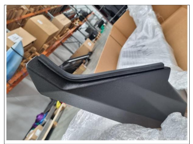
109. Fit the supplied lengths of side bulb pinch weld rubber to the outermost edge of the wing on each side of the bullbar.
