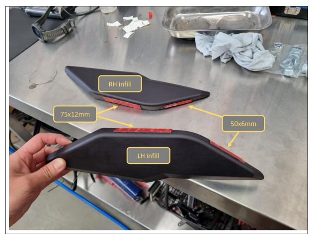
48. Apply 4x supplied 3M VHB tape strips to the 2x grille infills as shown.
