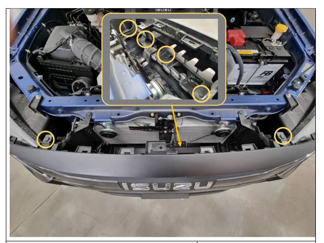
7. Remove 6x plastic push clips holding the grille.
